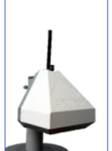
The AQMESH system will monitor the main gaseous emissions and particulates most commonly caused by shipping (NO; NO2; SO2; O3; PM10; PM2.5; PM1). Due to the lack of baseline data, we will be producing our own baseline for a period of 12 months to enable further analysis and comparisons to take place in the future. Data will be reviewed periodically to assess whether our strategies are effective at reducing the emissions output, both short, medium and long term.
