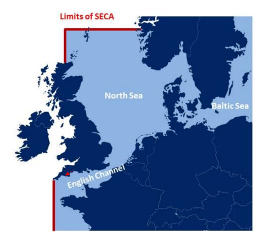
This means ships transiting through the English Channel, and into ports in this area, must burn fuel with a sulphur content lower than 0.1%. A study into shipping air quality by Plymouth Marine Laboratory has indicated that approximately 95% of ships in the Plymouth area are compliant with this sulphur limit. Where ships cannot switch to the low sulphur fuel, they are required to use other methods, such as scrubbers, to achieve the same effect.
