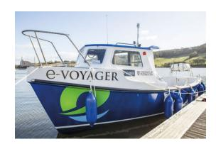
A vessel from the Mount Batten Ferry service fleet has had her engine replaced with a new electronic drive propulsion system and solar charging capability.
