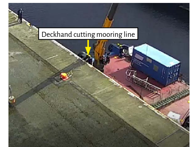
Figure 5: A deckhand cuts the forward mooring line, returning the vessel upright
