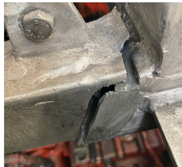
Figure 3: Fractured engine support
