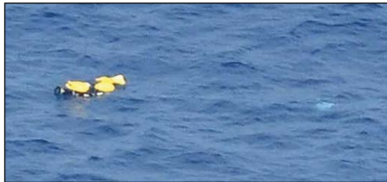
Figure 1: The port liferaft, floating inverted and partially inflated
