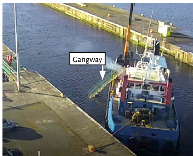
Figure 1: The workboat loses control of the gangway
