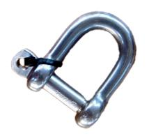
'Moused' shackle example. Cable tie/wire stops pin from working loose and dropping out and setting mooring rope/s free.
